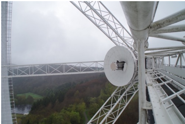
Fig. 1 The Phased Array Feed frontend installed at primary focus of Effelsberg 100m telescope.
